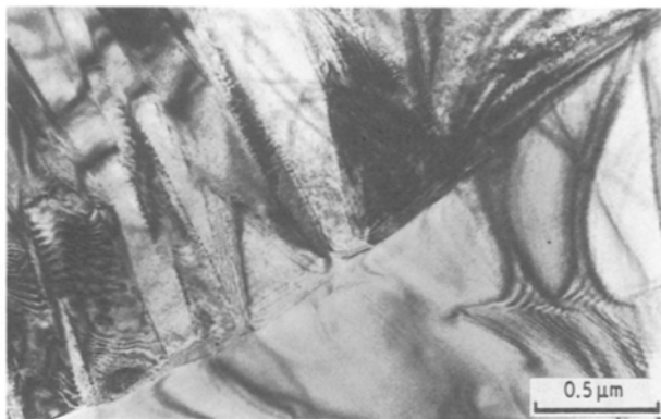
Figure 6 Photomicrograph Ce-TZP + Mn showing twins formed during the TEM analysis.
