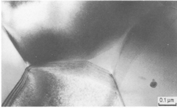
Figure 5 Transmission electron micrograph of Ce-TZP + Cu material showing a glassy phase pocket at the triple point.
